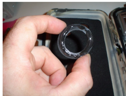
Figure 34 – Apply Marine GOOP to Flash Gasket
