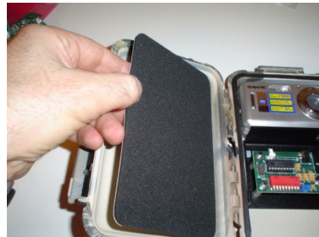
Figure 22 – Place foam insert into lid, do not stick into place
