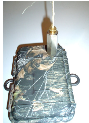
Figure 17 – Mark the location of the camera lens
