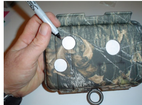
Figure 23 – Close lid 1/2 way and mark locations with fine tipped pen.
