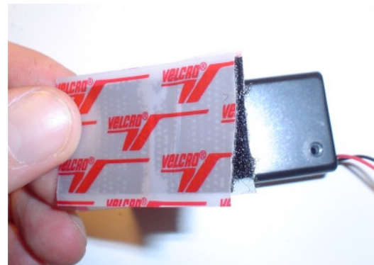
Figure 41 – Affix Velcro with adhesive backing to the back side of the battery holder case
