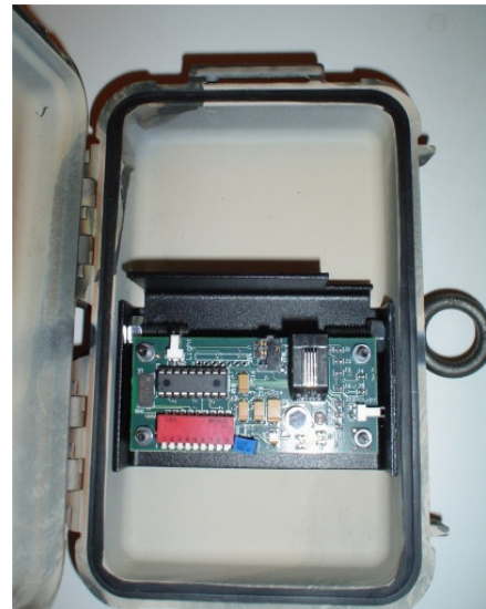
Figure 14 – Install both eye-bolts with Universal Board and metal fixture
