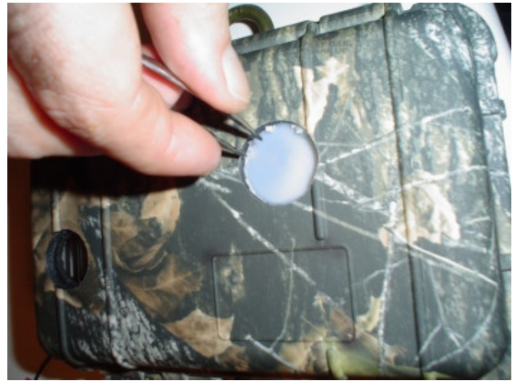
Figure 31 – Remove Marine GOOP after drying
