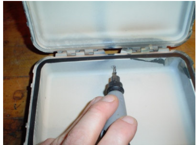
Figure 12 – Drill a small pilot hole
