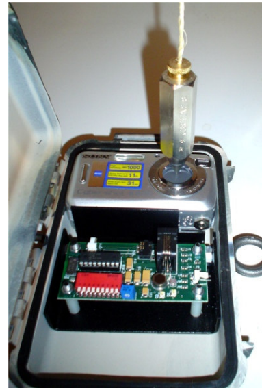
Figure 16 – Hang plumb bob above camera lens
