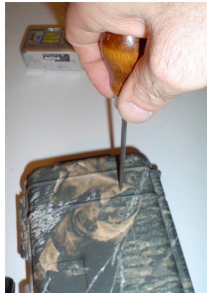
Figure 19 – Use an awl or center punch to prep hole for drilling
