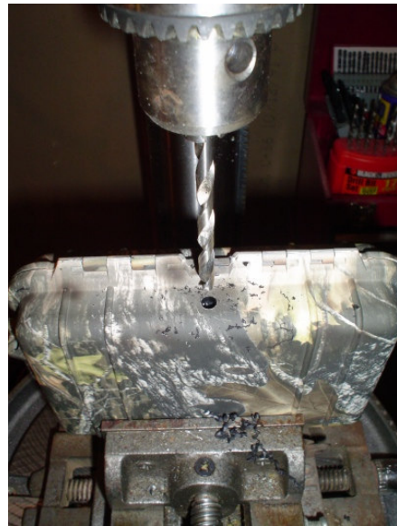
Figure 13 – Drill 1/4" hole for second eye-bolt
