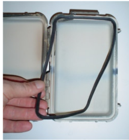
Figure 5 – Insert O-Ring into case tray groove
