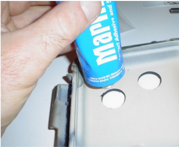
Figure 29 – Place Marine GOOP around the holes
