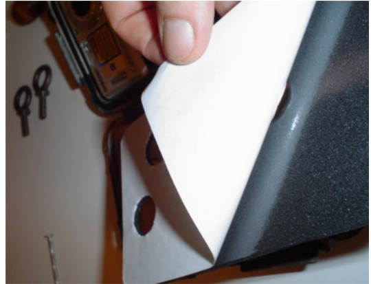
Figure 32 – Remove white paper backing from foam lid insert
