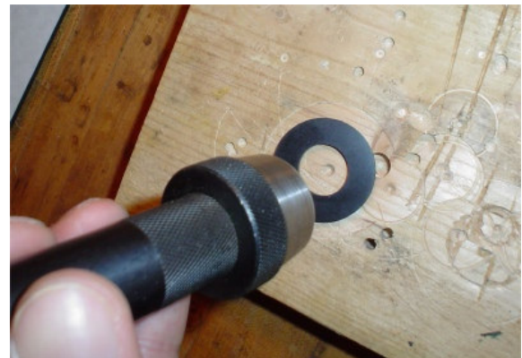
Figure 27 – Enlarge hole in flash masking gasket
