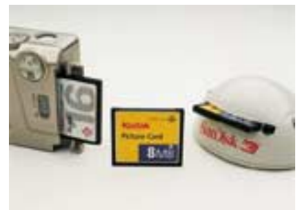
Flash Card Removable Media. On the left, a card is seen partially inserted into a digital camera. On the right is a flash card reader that can be attached to a computer for direct access to the images on the card.
