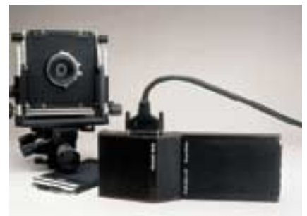
Digital Back for Use in a 4 \times 5 View Camera. The digital back is inserted into the camera where film holders would normally be placed.
