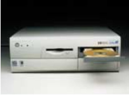
Computer. This case contains the CPU, a hard drive, a CD-ROM drive, and other electronic control circuitry.
