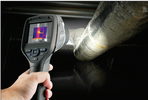
Built-in LED lamp lights dark areas for better digital images and safety.
