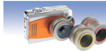
Digital camera with lenses modified to mount on microscope.
