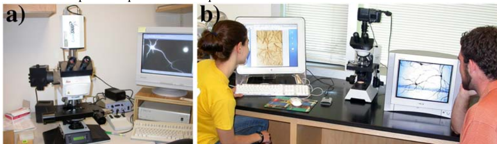
Fig. 1 A comparison between a) a research microscopy workstation and b) an inexpensive student workstation illustrates how the essential components of the research grade setup can be emulated to achieve a student grade digital microscopy workstation.
