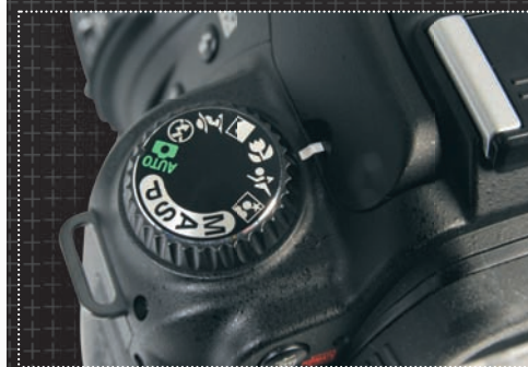
▲ These are not ordinary subject programs. No, they're 'Advanced Scene Modes' which not only optimise the exposure settings but also the digital imaging processing parameters.
