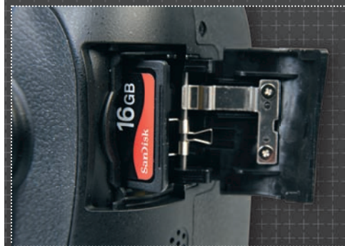
▲ The D90 accepts SD/SDHC memory cards and is the highest spec Nikon D-SLR to do so to date. However, with this format now matching CompactFlash cards for capacity and speed it's certainly not a problem.
