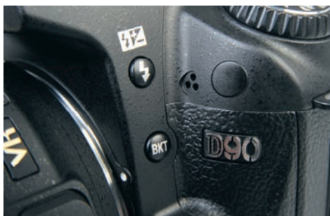
▲ A mono microphone is built into the front of the camera, but it has a severely limited dynamic range and there appears to be no way of connecting an external mic.
