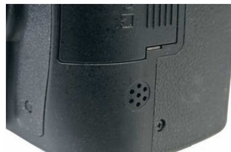
▲ The D90 has a loudspeaker built into the base of the handgrip for in-camera playback of movie clips.
