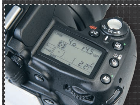
▲ The D90 has both front and rear input dials which are used in conjunction with the various function buttons for changing settings.
