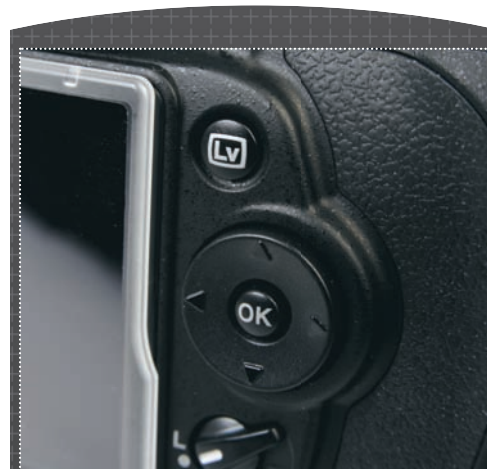
▲ Live view is activated by simply pressing the 'Lv' button on the camera's rear panel. This also readies the D90 for recording movies which are started and stopped by pressing the 'OK' button.
