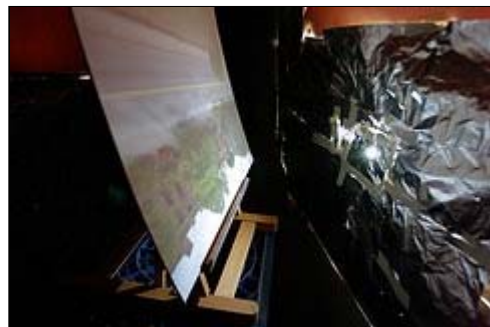
Fig 1.1.5 A camera obscura made by blocking a window. Photo by brighterorange , used under creative commons .
