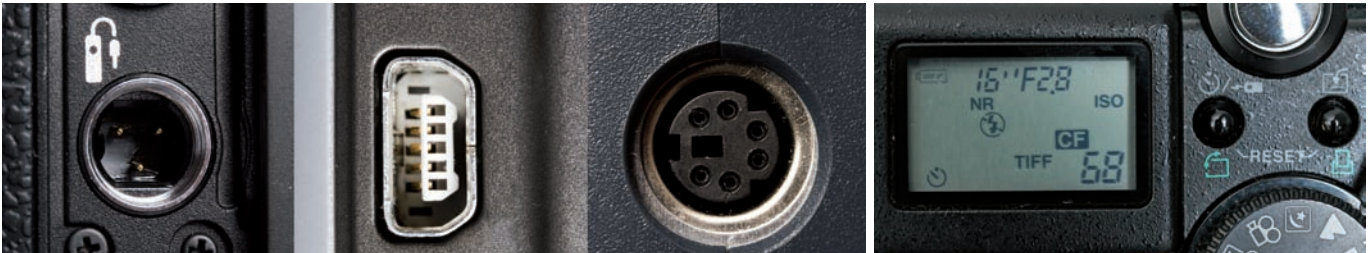
Connector sockets for remote control releases of different compact cameras.
