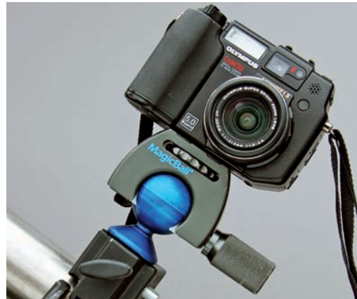
Camera with clamp and ball head on the counterweight bar of a telescope.
