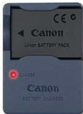
Battery in charger (can be plugged into an electrical outlet to charge). When the battery is fully charged the light will turn green.
