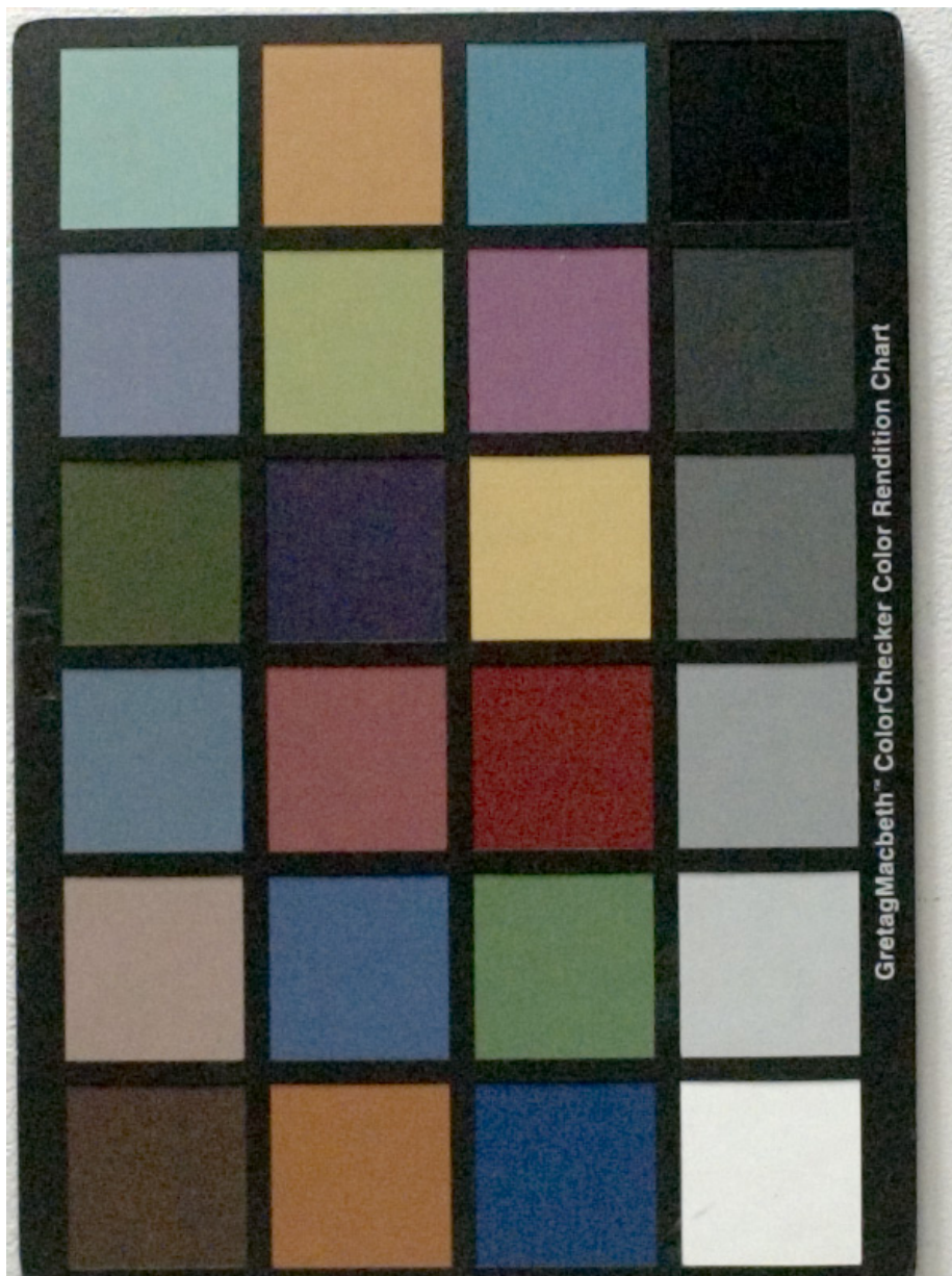
Figure 11: V7.3 color exposed for ISO 11000. This is the same image as the previous one, with color noise reduction applied (33 in Adobe Camera Raw™). Image sharpness is not affected, and noise is less noticeable.
