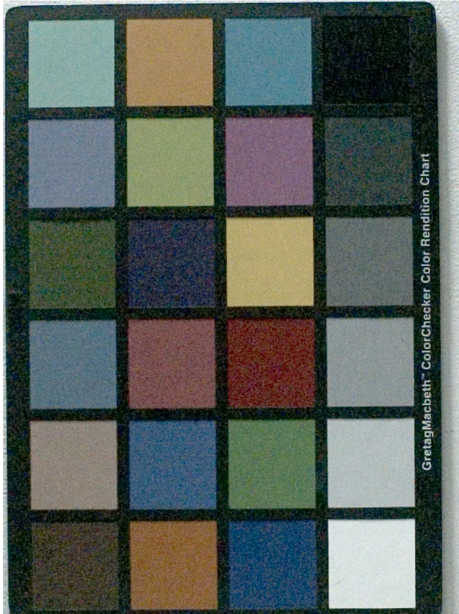
Figure 12: V7.3 color exposed for ISO 22000. Signal to noise ratio of the 19% gray patch (third from the right) is 4. Overexposure latitude is 4.5 stops.
