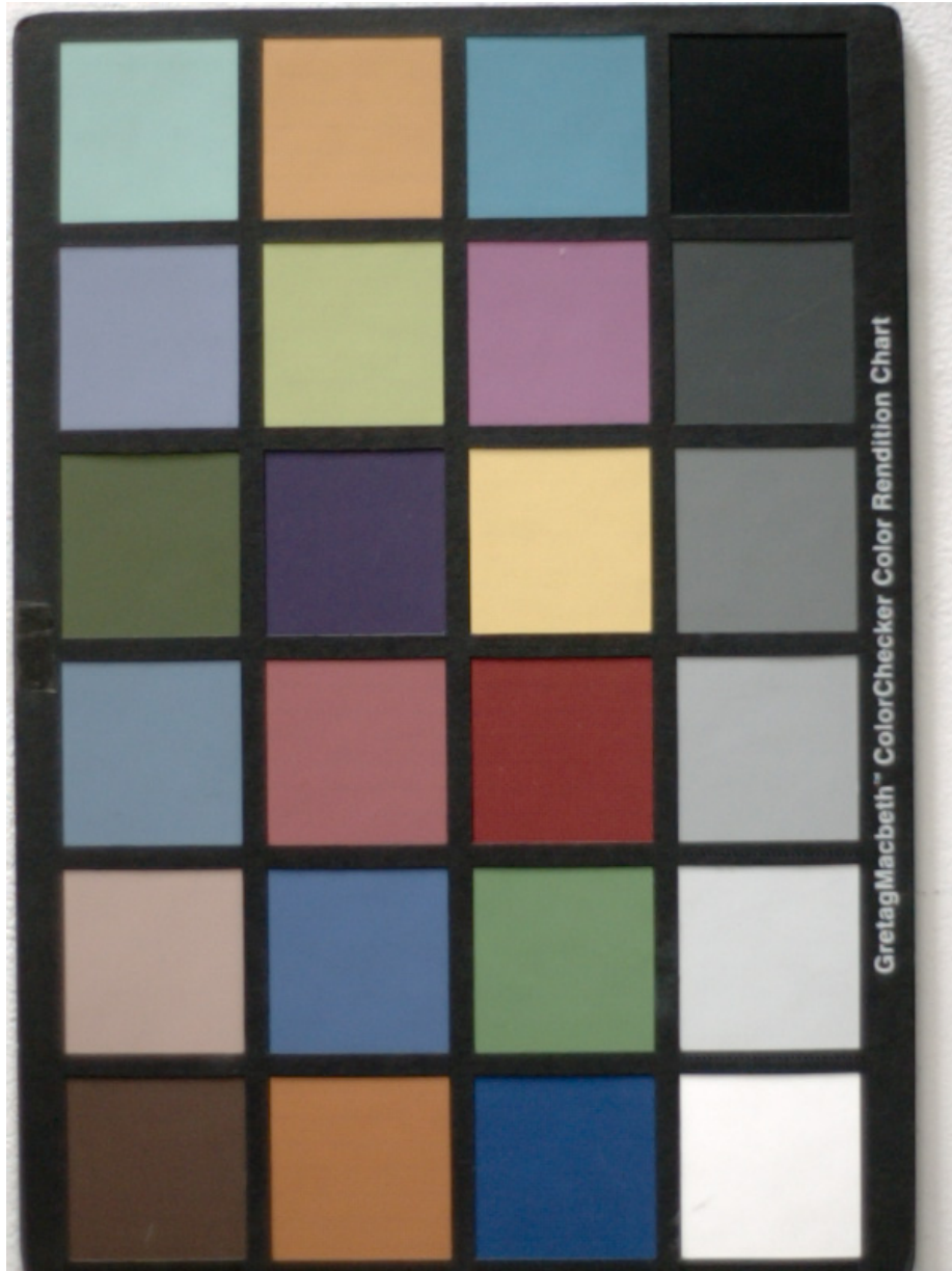
Figure 6: V7.3 color exposed for ISO 1400. Signal to noise ratio of the 19% gray patch (third from the right) is 47. Overexposure latitude is 0.5 stops. This would be the saturation-based iso setting when white-balanced for daylight.
