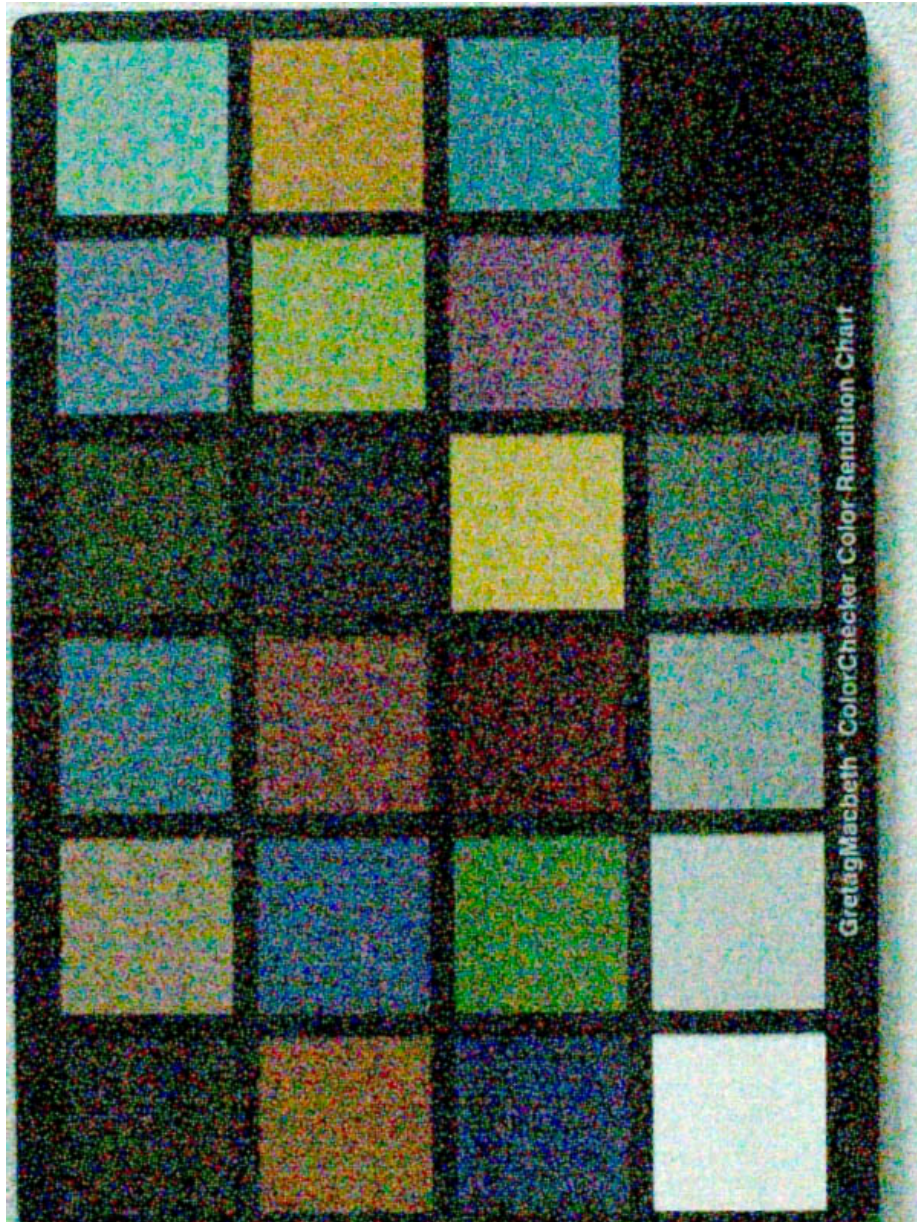
Figure 14: V7.3 color exposed for ISO 88000. Signal to noise ratio of the 19% gray patch (third from the right) is 1. Even at this high noise level, the contour of the patch can be easily discerned. Reading the small text on the chart is easy. The 9% patch (second from the right) reflects only 1/900 of the light needed to saturate the sensor.
