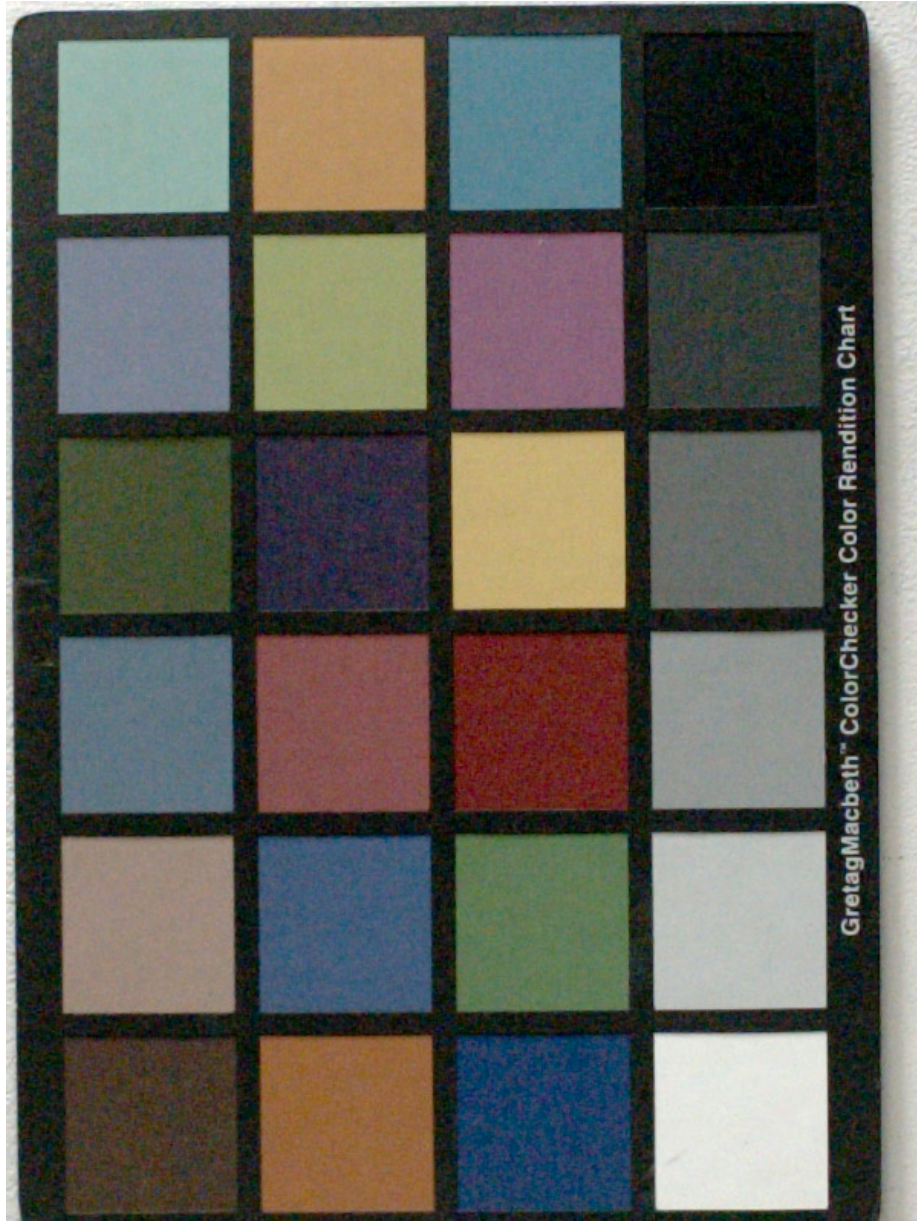
Figure 10: V7.3 color exposed for ISO 11000. Signal to noise ratio of the 19% gray patch (third from the right) is 10. This is the “first acceptable” illumination level. Overexposure latitude is 3.5 stops.
