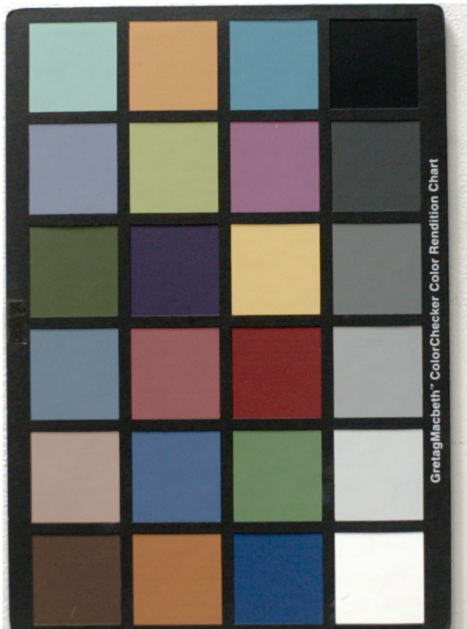
Figure 7: V7.3 color exposed for ISO 2800. Signal to noise ratio of the 19% gray patch (third from the right) is 30. Overexposure latitude is 1.5 stops.
