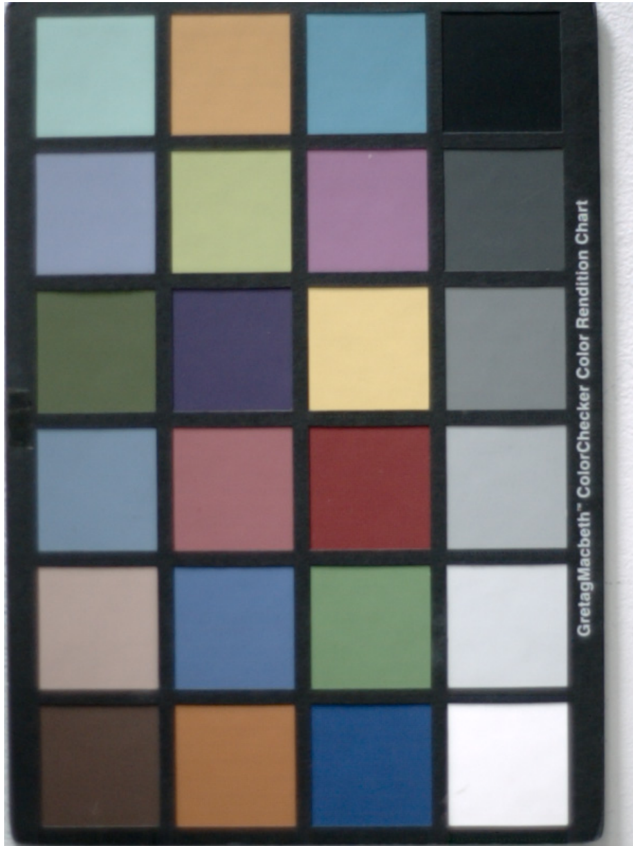
Figure 5: V7.3 color exposed for ISO 1200. Signal to noise ratio of the 19% gray patch (third from the right) is 60. Overexposure latitude is zero. With naturally-balanced light, at this EI the overexposure latitude would be 1/4 stops; however, balancing the for the test lighting (daylight) used up that latitude.
