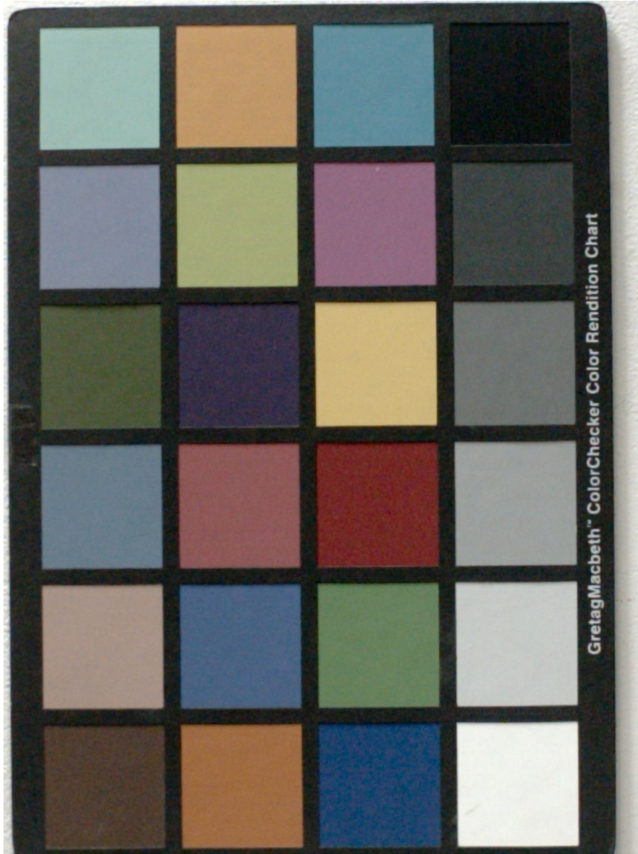
Figure 8: V7.3 color exposed for ISO 5600. Signal to noise ratio of the 19% gray patch (third from the right) is 18. Noise beginning to be apparent on the darker patches. Overexposure latitude is 2.5 stops.
